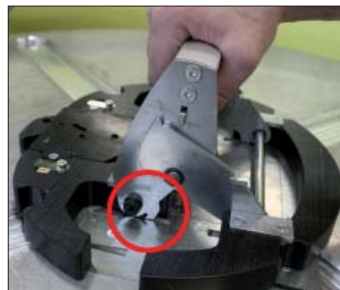
Collapsed center - Releasing the hooks from the plate
