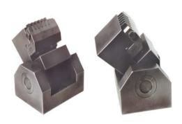
Grinding fixture for setting tools, single as well as multiple, type 602, 603, 604 and 605.
