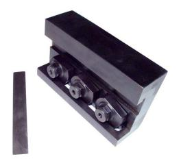
Grinding fixture for setting tools, mainly for tools type 606 and 607, shorter tools can also be regrinded in this fixture.
