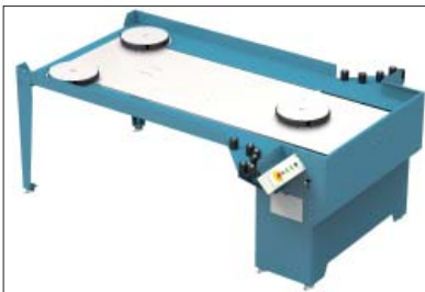
The band loop generate a loop of band, this will give time to weld coils together. Picture 3
