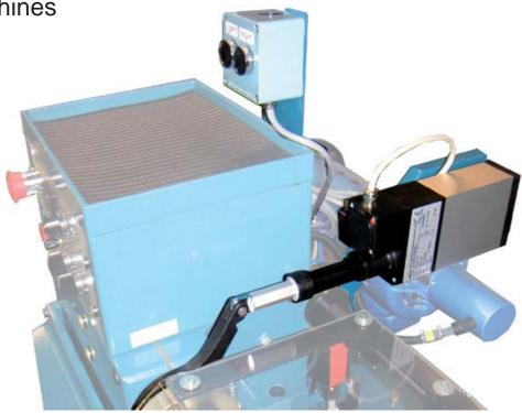
The most frequent and most important set adjustment when setting a band saw is the symmetry adjustment. The new versions of the SGS software (5.01 and later) will now allow the ALO 185 set gauge to control the set symmetry and continuously make adjustments by means of a servo motor. This will give you advantages such as less stops for operator adjustments, possibility to keep a tighter symmetry / balance tolerance on your bands, and a lower scrap percentage due to miss adjustments.
