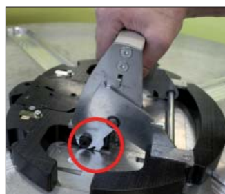
Collapsed center Equipped with a safety lock
