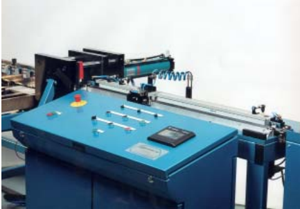
Feeding system with programmable linear feeder.
