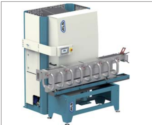
High velocity nitrogen gas quenching zone. Picture 7
