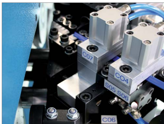
Shear and strip feeding unit.
