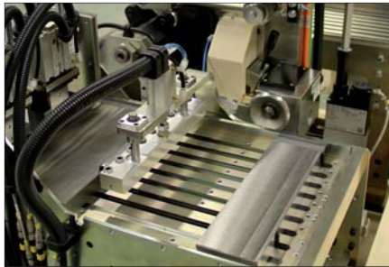
Infeed magazine ready to fill up the batch with a new blade package.
