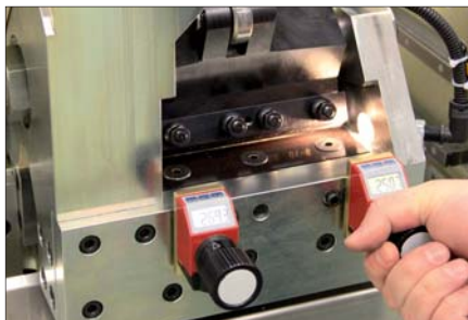
Improved clamping together with digital micrometer makes clamping adjustments easier.
