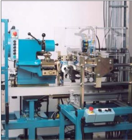
Pick and place unit and setting unit
