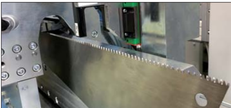
Laser sensor tooth positioner and setting unit
