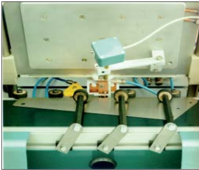
Hardening inductor with flash guard and air quench
