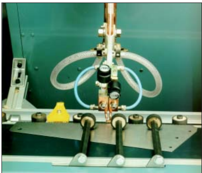
Tempering inductor and air cooling
