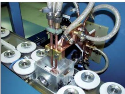
Feed unit, hadening coil and quenchant chamber
