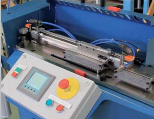
The feeding system with clamping jaws on each side.
