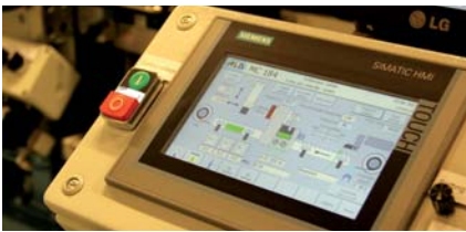
Operator friendly HMI gives full control of the setting operation.
