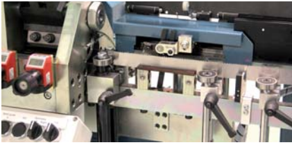
New programmable linear servo carry out the feeding of the blade.
