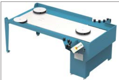
The band loop generate a loop of band, this will give time to weld coils together. Picture 3
