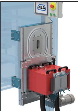
The work coils can be lowered out of the way to a service pos.
