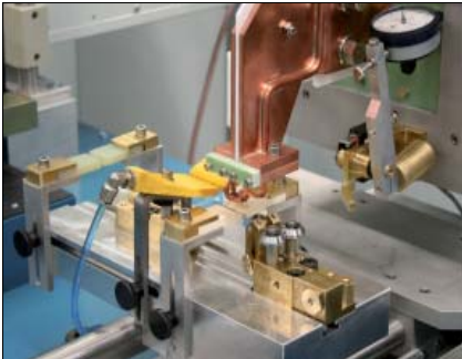
Tooth hardening inductor with air quench
