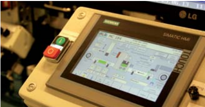
Operator friendly HMI gives full control of the setting operation.
