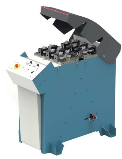
The ALO 200844 is a twin feeding station that uses two separate 6 wheel feeding units. The feed units has separate motors and they run separate from each other.
