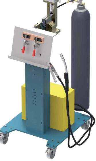
This system contains a band weld fixture and a pneumatic shear to trim the ends of the bands before welding them together in the fixture for continuous hardening/tempering.
