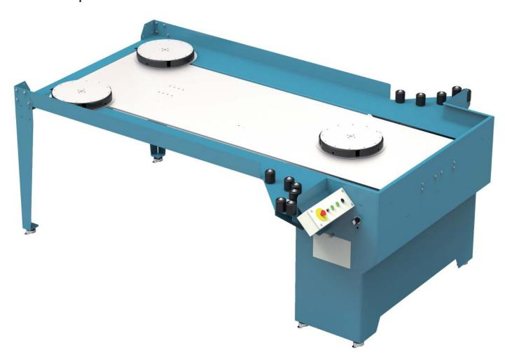
The band accumulator can be activated to generate a 12m loop of band at any time. When it's time to change coiler or cube the band end is locked and band is automatically fed into the loop accumulator allowing time to change coiler or cube. This will give time to weld coils together and facilitate continuous hardening/tempering. After welding, the band loop has been consumed allowing band to be feed directly from coiler or cube system again.
