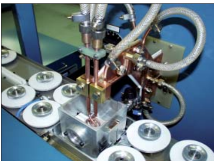
Feed unit, hadening coil and quenchant chamber
