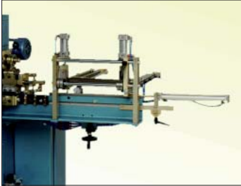
Feed magazine will separate and feed one blade at a time to the setting unit.
