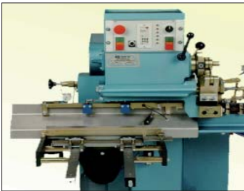
Feed and screw collector magazine will stack up to 700 blades.
