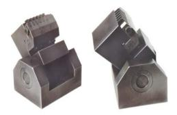
Grinding fixture for setting tools, single as well as multiple, type 602, 603, 604 and 605. The fixture has a fixed position for grinding of the carbide height as well as scale marks 0-30° for grinding of the angle.
