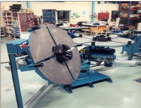
*Picture showing tilt able take up coiler*
