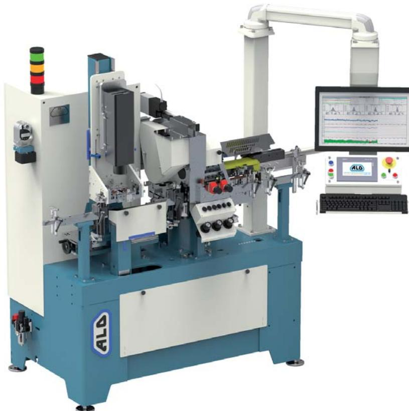
The new generation ALO setting machine that together with the SGS camera system will help you to monitor and get in full control of the setting process and quality.
