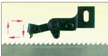
The feeding device does not come in contact with the tooth tip. The feeding pin is made of hard metal and interchangeable to match different tooth forms.
