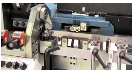
New programmable linear servo carry out the feeding of the blade.
